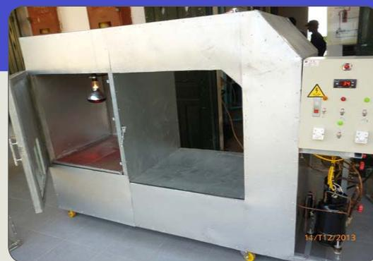
In addition, this design can automatically adjust the drying temperature from 20°C to 60°C, depending on technology requirements; Based on the convection or fluidized bed drying model, the wind speed entering the drying chamber can vary between 0.5 - 1.2m/s; The distance from infrared light to the drying material is around 20 - 50 cm.
